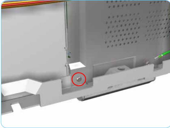
6. Remove 1 T-10 screw securing the Plastic Cover. Remove the Plastic Cover from the Printer.
