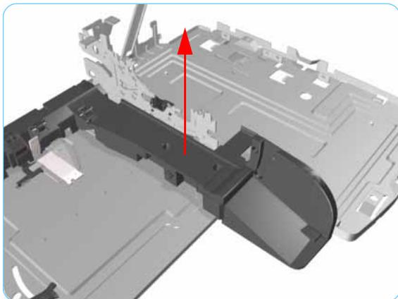
20. Lift the Right Bracket out of the Printer.
