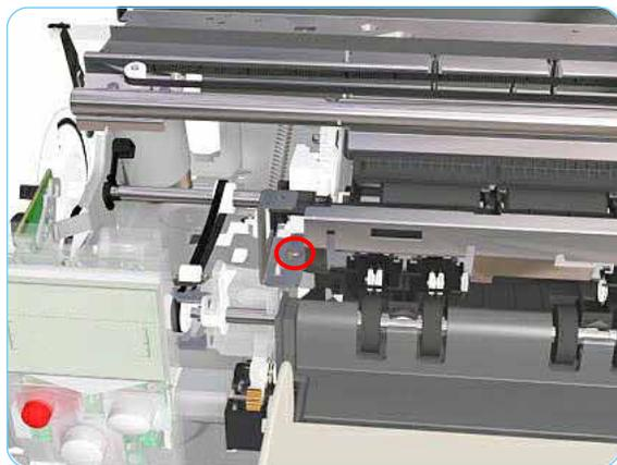
3. Remove 1 T-10 screw (**Type A**) that secures the Starwheel Assembly to the left hand side of the printer.
