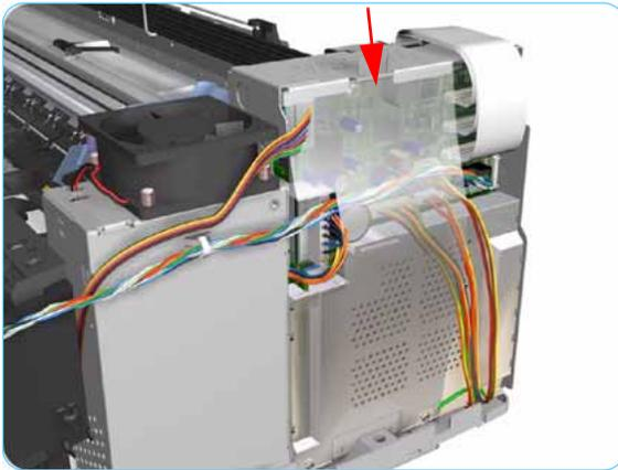
3. Release the Plastic Cover protecting the Electronics Module.
