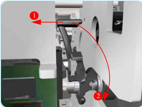
4. Raise the locks so that they are aligned with the cutouts and lift out the Pick Assembly from the Printer.
