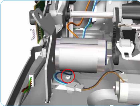
12. Remove 1 T-10 screw that secures the Paper-Axis Motor Mount.
