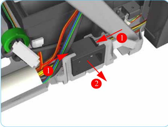
6. Press in the clips on either side and release the Power Socket.
