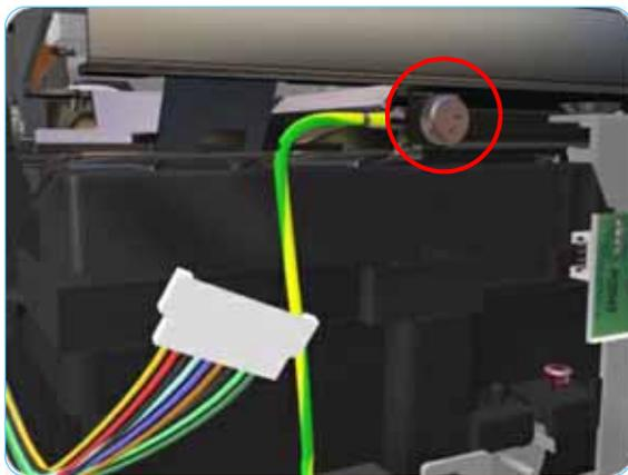
5. Remove 1 T-10 screw (**Type A**) that secures the Grounding Strip.
