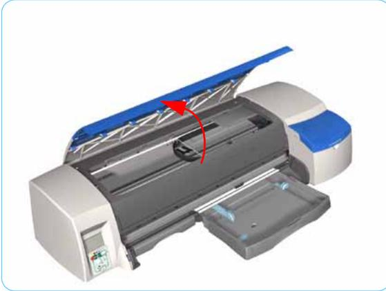
2. Release the clips that secure the Top Cover and remove from the Printer.
