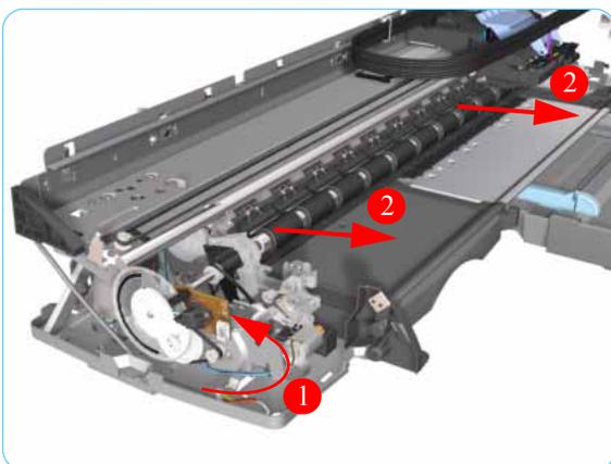
21. Raise the locks so that they are aligned with the cutouts and lift out the Feed Roller Assembly (including the Paper-Axis Motor) from the Printer.
