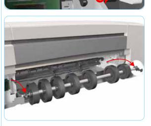
4. Raise the locks so that they are aligned with the cutouts and lift out the Pick Assembly from the Printer.
