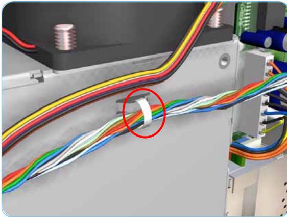
7. Cut the Plastic Tie that secures the Ink Supply Station Cable to the Power Supply Unit.
