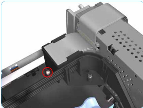
4. Remove 1 T-10 screw that secures the Trailing Cable Support to the Carriage Assembly. Release the Trailing Cable Support from the Carriage Assembly.
