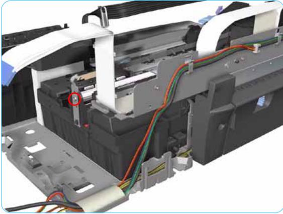
10. Remove 1 T-10 screw that secures the Encoder Strip Holder on the right hand side of the Printer.
