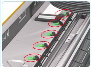
5. Release ALL the Pinch Springs from the Pinch Assembly.
