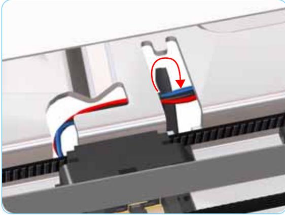
6. Release the Out-of-Paper Sensor cable that is looped underneath the Pinch Assembly.
