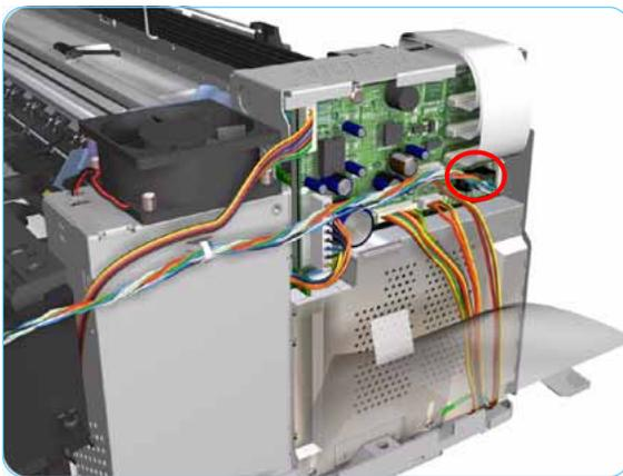
5. Disconnect the Ink Supply Station Cable from the Main PCA.
