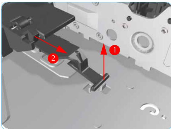
22. Remove the Bypass Platen Actuator from the Printer.
