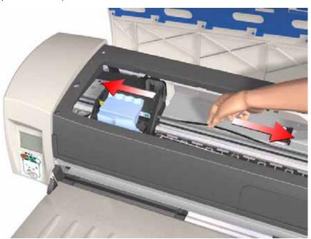
5 Using the belt, move the Carriage Assembly backwards and forwards over the Pivot Assembly (but staying on the left hand side of the printer), carefully listening for a scraping sound.
