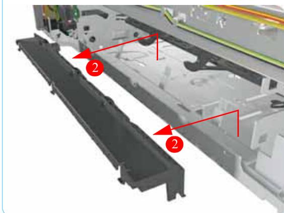
4. Remove the Lower Paper Guide from the Printer.
