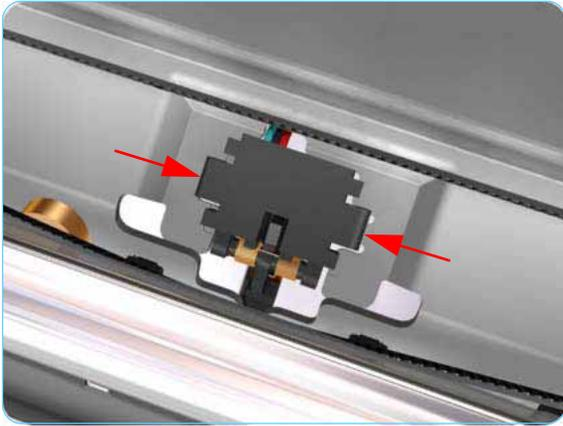
8. Press the OOPS Sensor clips inwards to release it.
