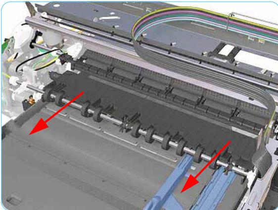
10. Slide out the complete Output Mechanism Assembly.
