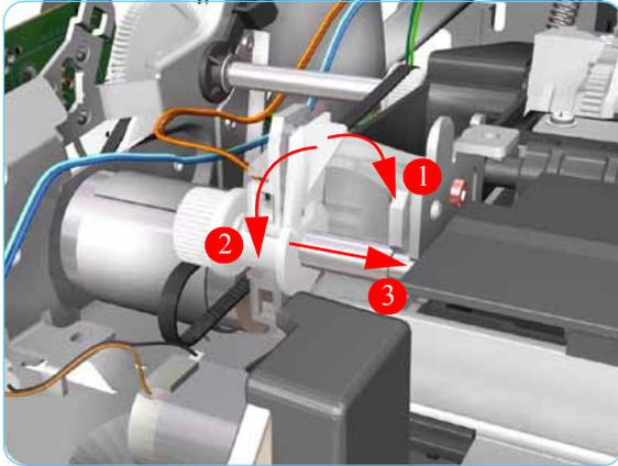
7. Release the locking mechanism from the left hand side of the Printer.
