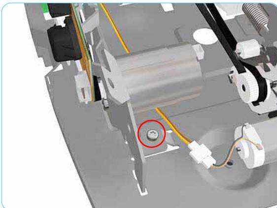
5. Release the locking mechanism that secures the Paper-Axis Motor Mount.
