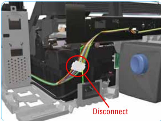
4. Disconnect the Motor Harness Cable.
