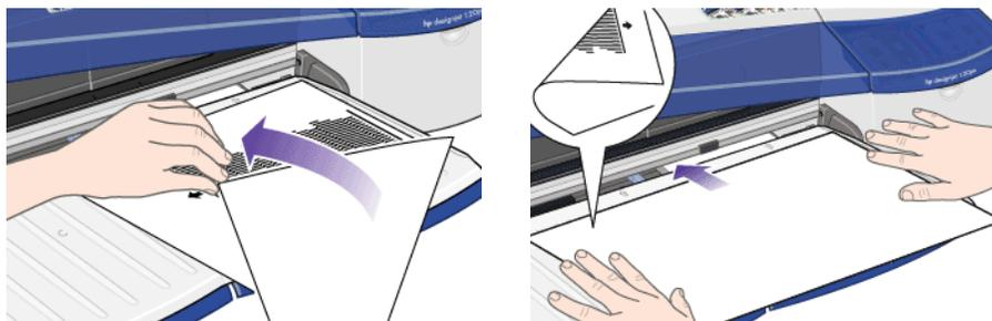
**Step 1** - Rotate the page and reload it upside down (image facing down)
