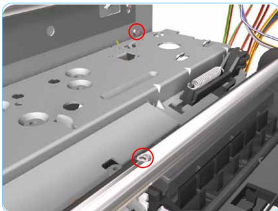
**17.** Remove 2 screws that secure the Hanger Assembly on the right hand side of the Printer.
