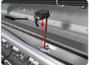
8. Press the 0 OPS Sensor clips inwards to release it.
