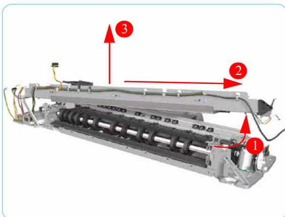
22. Remove the Hanger Assembly from the Printer.
