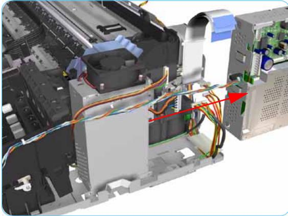
11. Remove the Electronics Module from the Printer.
