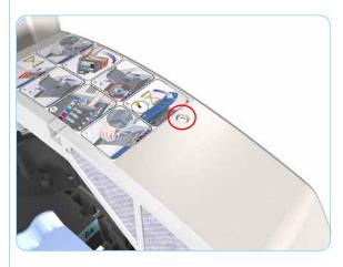
4. Remove 1 T-10 screw that secures the Right End Cover to the Printer.
