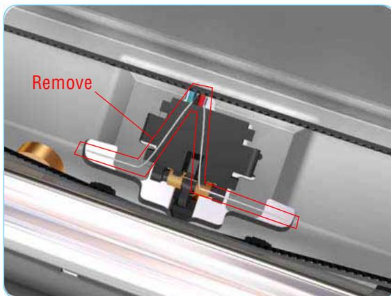
7. Remove the Spring that secures the O OPS Sensor.
