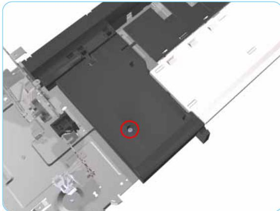
**20.** Remove 1 T-10 screw that secures the Side Guide to the Chassis.
