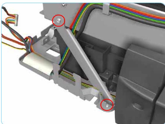
5. Remove 2 screws that secure the Reinforcement Bracket. Remove the Reinforcement Bracket from the Printer.
