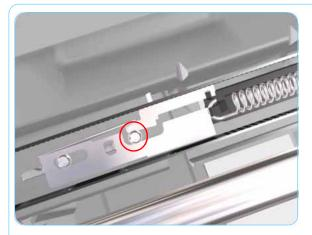
3. Insert the 2nd screw (right) and tighten it. As you tighten the screw you should notice that the slot in the Stopper will rise away from the Turnaround Assembly.
