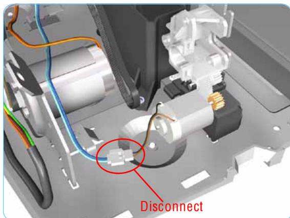
7. Disconnect the Ramp Motor cable.
