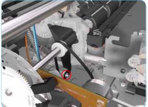
**15.** Release the locking mechanism from the right hand side of the Printer.
