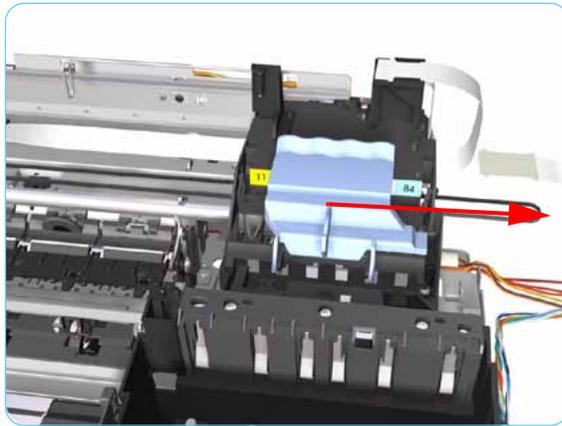
13. Slide the Carriage Assembly to the right and out of the Printer.
