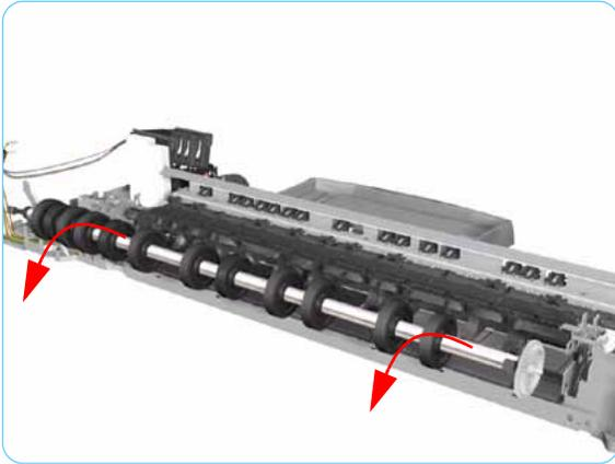
25. Raise the locks so that they are aligned with the cutouts and lift out the Pick Assembly from the Printer.
