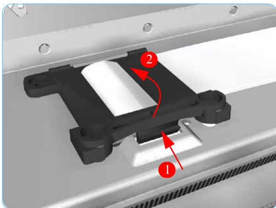
10. Release the Trailing Cable Clip from the Chassis.
