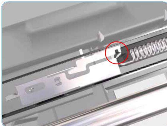
1. Place the Turnaround Stopper in to position and locate the slot in the Stopper on to the Turnaround Assembly. This step is very important since it will determine the space between the Stopper and the Turnaround Assembly.
