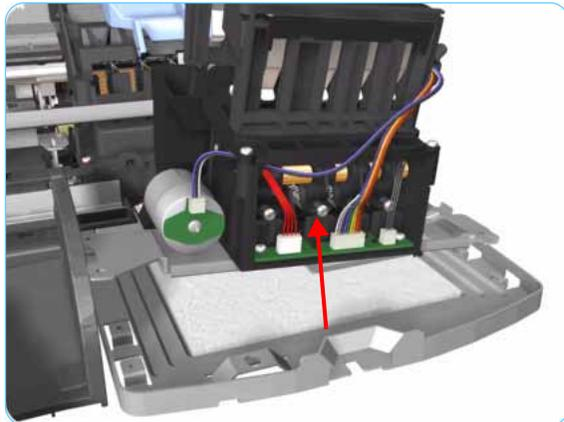
**11.** Remove the Ink Supply Station from the Printer.
