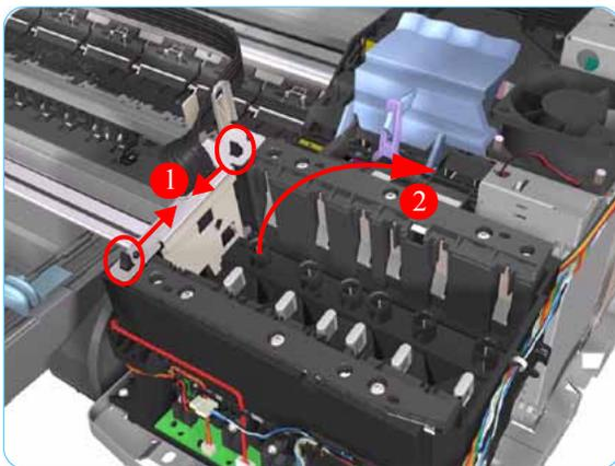
8. Release the Tubes Bracket from the Ink Supply Station by pushing the clips inwards and lifting up the Bracket.
