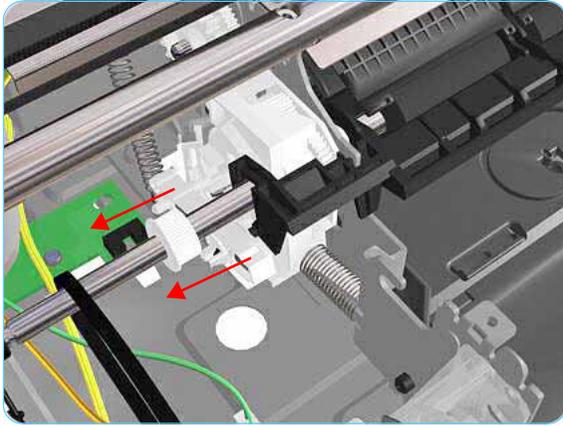
12. Release the Pin Caber and remove from the Printer.
