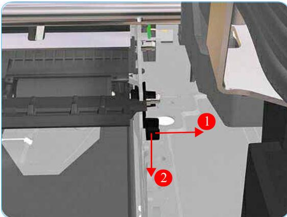
11. Release the locking mechanism from the right hand side of the Printer.
