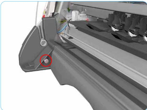
5. Remove 1 T-10 screw from the Left Side Bracket.
