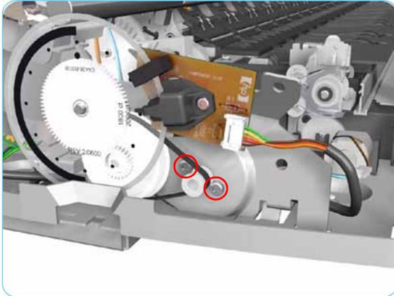
4. Disconnect the Paper-Axis Motor cable.
