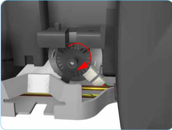
7. Uncap the Carriage Assembly by turning the Service Station Motor clockwise.
