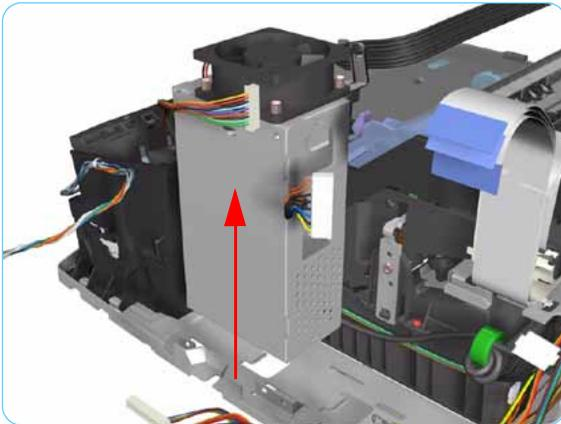
7. Remove the Power Supply from the Printer.
