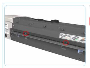
5. Remove 2 T-10 screws that secure the Center Cover from the rear.
