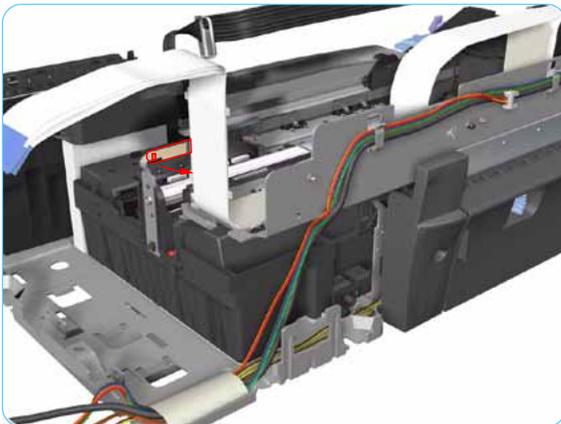
9. Release the Encoder Strip from the Encoder Strip Holder.
