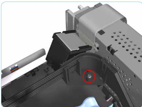
5. Remove 1 T-10 screw that secures the Tube Crane to the Carriage Assembly.
