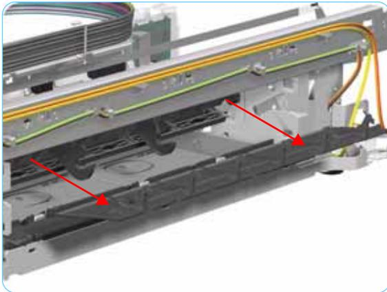
7. Working from the rear, pull out the Pinch Assembly from the Printer.
