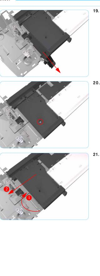
**19.** Slide the Left Bracket out of the Printer.
