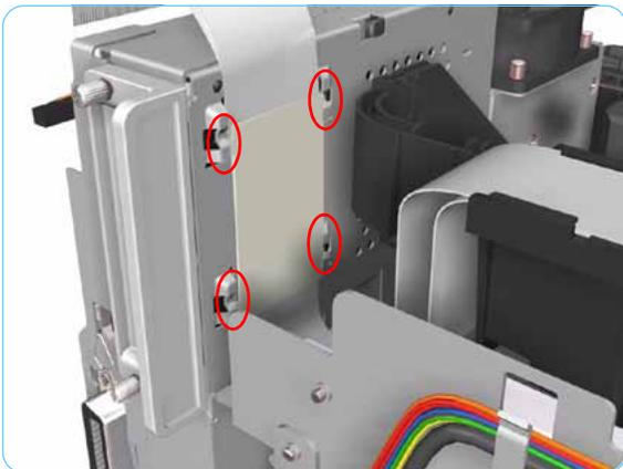
8. Release the plastic sheet that secures the Trailing Cable to the back of the Electronics Module.
