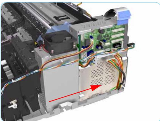
9. Slide out the Electronics Module and the Power Supply Unit (as one assembly) to the right.
