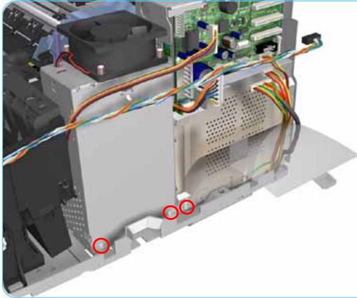
5. Remove 3 T-10 (**Type B**) screws that secure the Electronics Module and the Power Supply Unit to the Printer.
