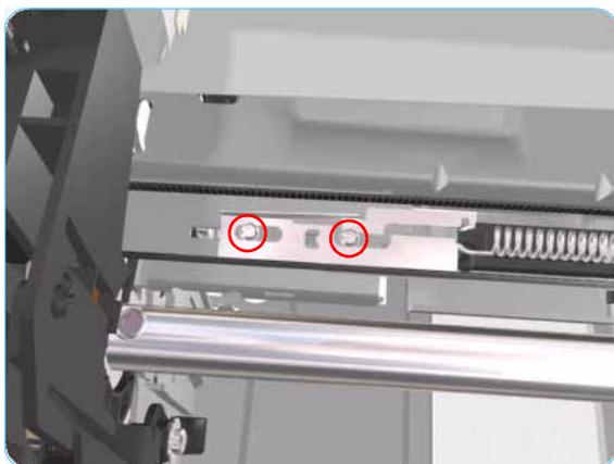
11. Remove 2 T-10 screws that secure the Turnaround Stopper. Remove the Turnaround Stopper from the Printer.
