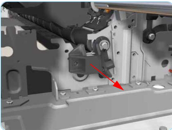
14. Remove the Pivot Assembly Support from the Printer.
