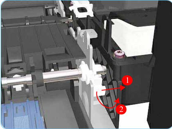
9. Release the locking mechanism from the right hand side of the Printer.
