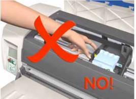
Incorrect: never move using Carriage Assembly.
