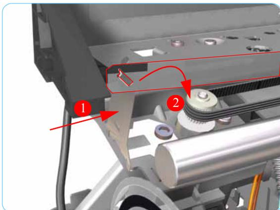
5. Release the Encoder Strip from the right hand side of the Printer.
