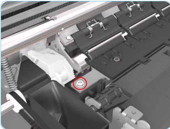
6. Remove 1 T-8 screw and washer that secure the Pivot Assembly on the right hand side of the Printer.
