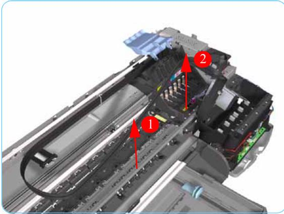
7. Lift up the Tube Crane (1) to release the PH Cover (2) from the Carriage Assembly and remove from the Printer.
