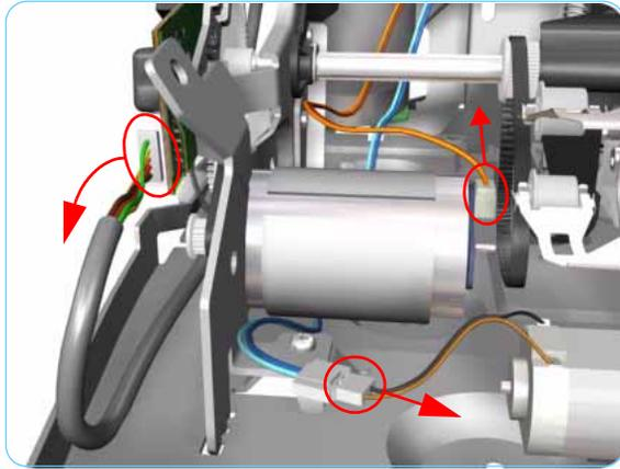
**13.** Disconnect the Paper-Axis, Encoder and Ramp Motor cables.
