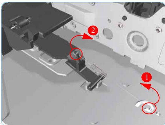
21. Release the Spring from the Bypass Platen Actuator.
