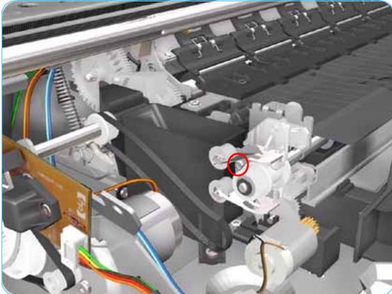
6. Remove 1 T-10 screw that secures the Spring Idler. Remove the Spring Idler from the Printer.
