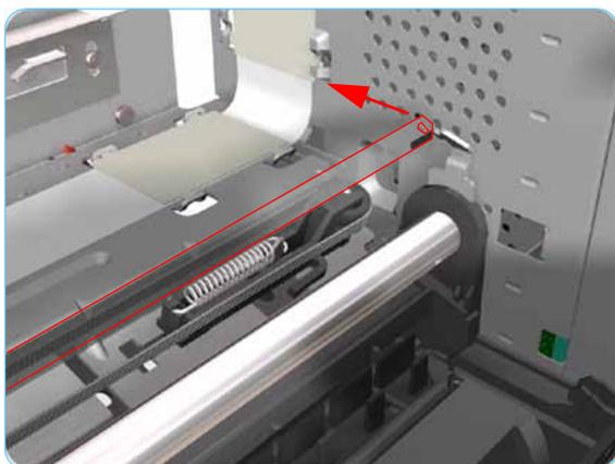
6. Gently slide out the Encoder Strip through the Carriage Assembly and remove from the Printer.
