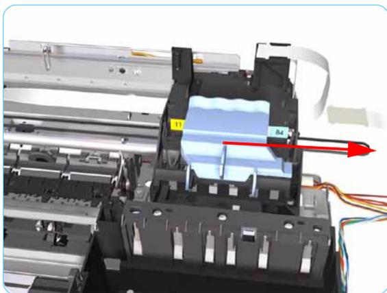
12. Slide the Carriage Assembly to the right and out of the Printer.
