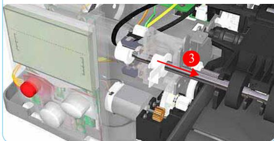
8. Release the locking mechanism from the left hand side of the Printer.
