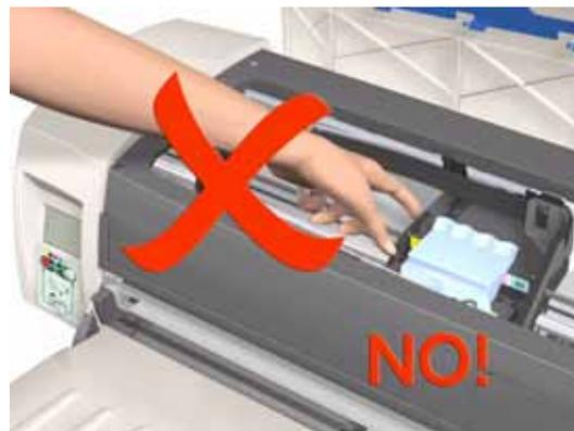
**Incorrect:** never move using Carriage Assembly.
