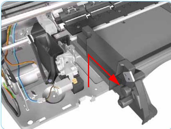
6. Remove the Front Left Bracket from the Printer.
