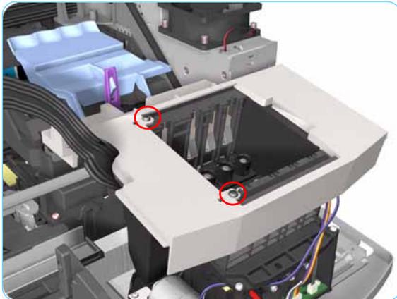
5. Remove the ISS Cover from the Printer.
