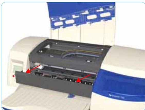
3. Remove the Front Cover from the Printer.
