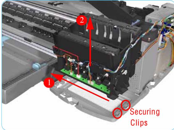
**10.** Move the Ink Supply Station to the left to release it from the securing clips.
