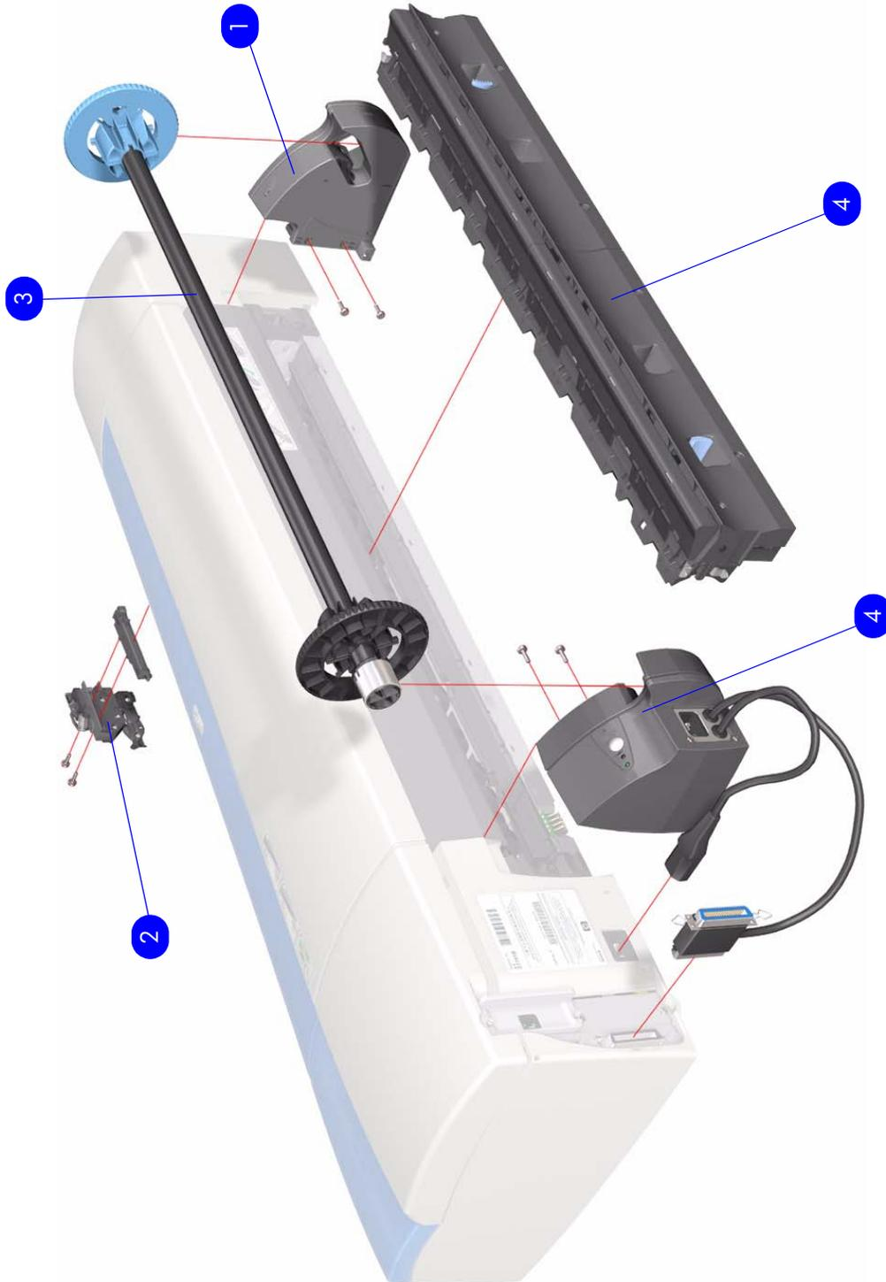
**Figure 16: Rollfeed Components**
