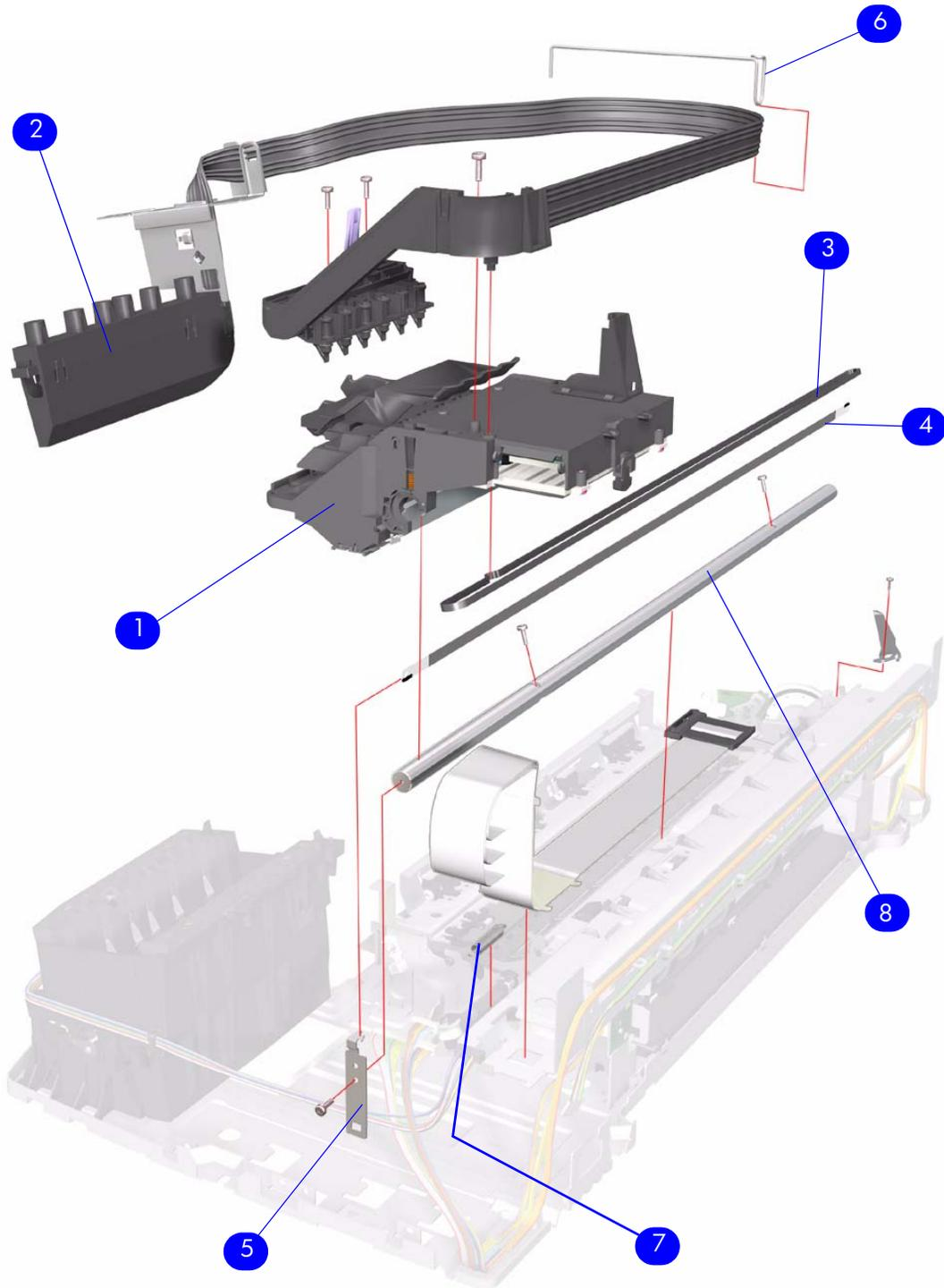
**Figure 6: Scan-Axis Assemblies**
