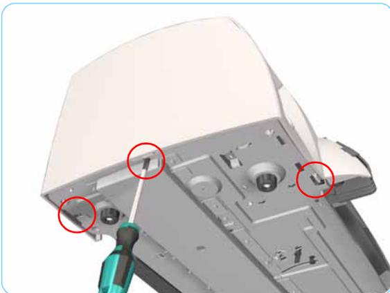
6. Release the clips that secure the Left End Cover to the Printer (use a flat-blade screwdriver if necessary).
