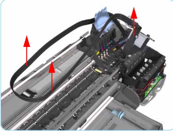
9. Release the Ink Supply Tubes and remove from the Printer.
