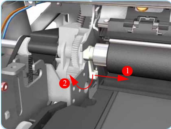
19. Release the locking mechanism from the left hand side of the Printer.
