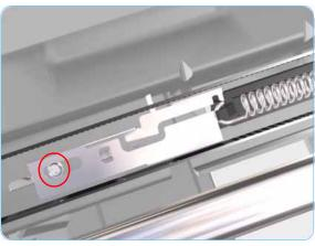
2. Insert the first screw (left) and tighten it.
