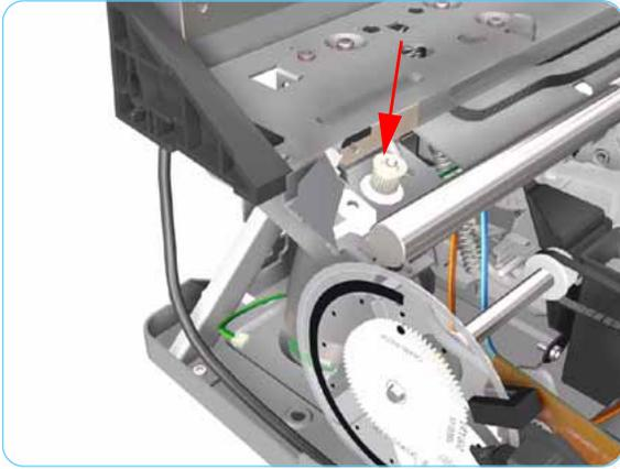
7. Remove the Carriage Motor from the Printer (needs to be removed from underneath).
