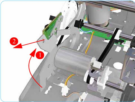
6. Remove the Paper-Axis Motor Assembly from the Printer.
