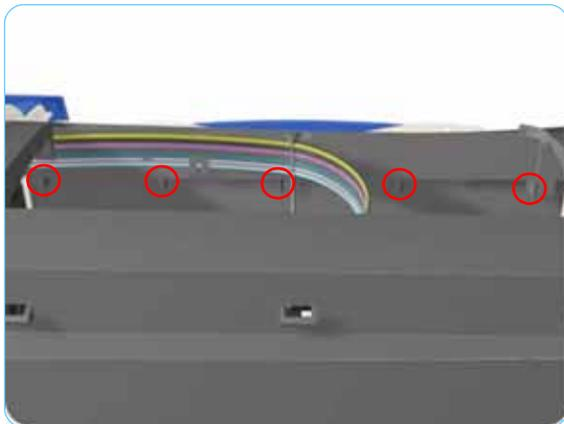
2. Release the clips (from the inside) that secure the Front Cover.
