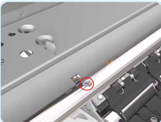
12. Remove 1 screw that secures the Hanger Assembly on the left hand side of the Printer.
