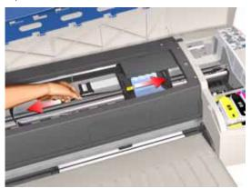
**10** Using the belt, move the Carriage Assembly backwards and forwards over the Pivot Assembly (but staying on the right hand side of the printer), carefully listening for a scraping sound.
