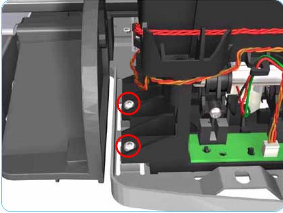
9. Remove 2 T-10 screws that secure the Ink Supply Station.
