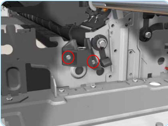
13. Remove 2 T-10 screws that secure the Pivot Assembly Support on the right hand side of the Printer.
