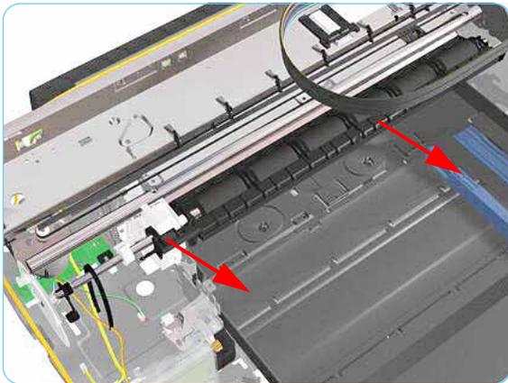
14. Raise the locks so that they are aligned with the cutouts and lift out the Feed Roller Assembly from the Printer.
