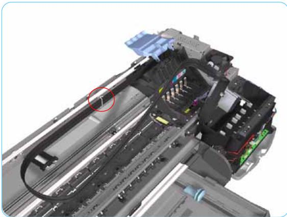
8. Release the Ink Supply Tubes from the Raceway Holder.
