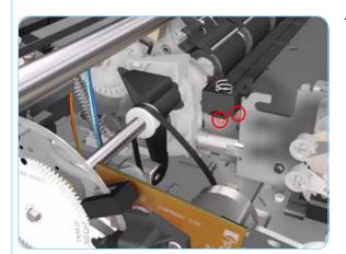
**17.** Remove 2 T-10 screws that secure the bracket on the left hand side of the Printer.
