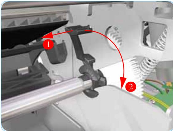
3. Release the locking mechanism that secures the Pick Assembly on the left hand side of the printer (looking from the rear)
