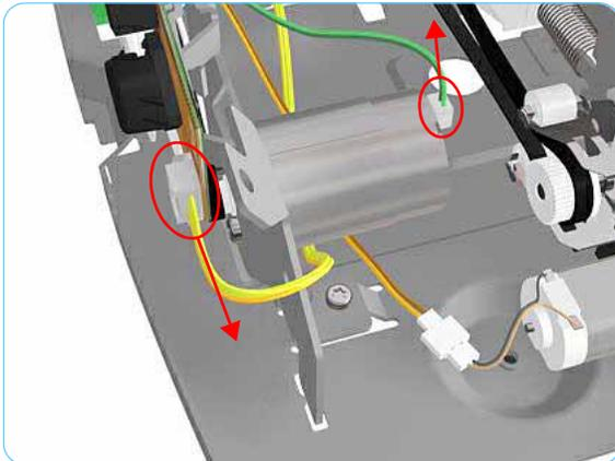
4. Remove 1 T-10 screw (Type A) that secures the Paper-Axis Motor Mount.
