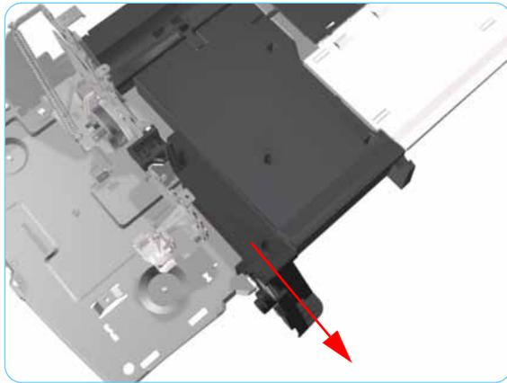
**19.** Slide the Left Bracket out of the Printer.
