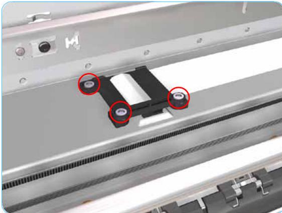
9. Release the Trailing Cable Clip from the Chassis.
