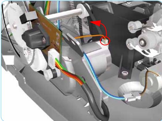
5. Release the belt from the Paper-Axis Motor. Remove the Paper-Axis Motor Assembly from the Printer.
