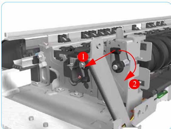
24. Release the locking mechanism that secures the Pick Assembly on the left hand side of the printer (looking from the rear)
