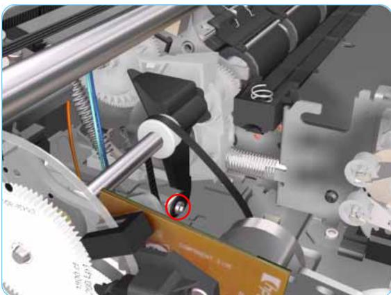
16. Remove 1 T-10 screw and nut that secures the Feed-Roller Support on the left hand side of the Printer.
